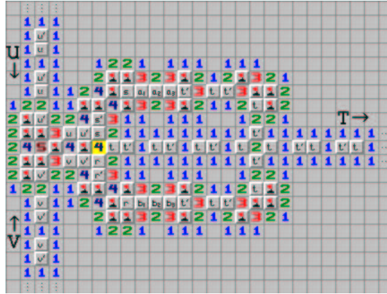
An AND gate translated into Minesweeper. A good Minesweeper player will never make a guess if there is a square that is certainly free and a guess is not required. Similarly he or she will mark up every mine that can be identified with certainty. [Fig. 4]
